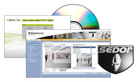
DVS Analysis Server is a SEDOR® video analysis server software for the analysis of up to 24 IP-based video streams. It is designed for the installation on dedicated and qualified server hardware and is configured with a browser over Ethernet using the integrated SEDOR® WebGUI. Together with the optional licenses for the various SEDOR® applications up to 24 channels can be used for video analysis according to demand.
